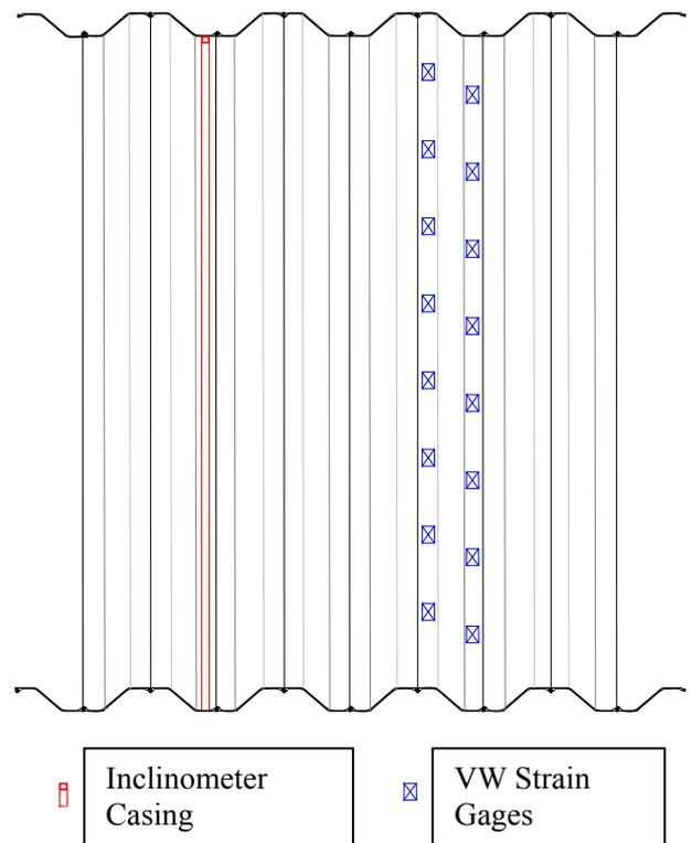
Figure 7. Strain gage and inclinometer layout
