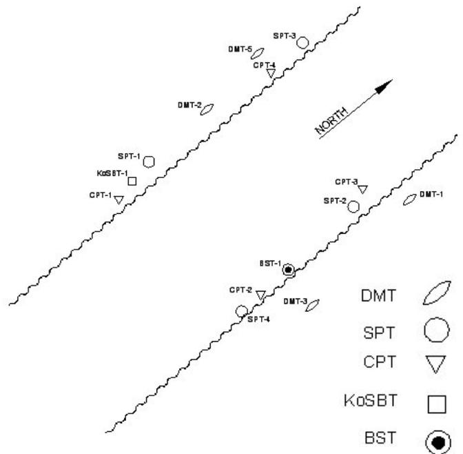
Figure 3 Layout of insitu tests at Statesville site
